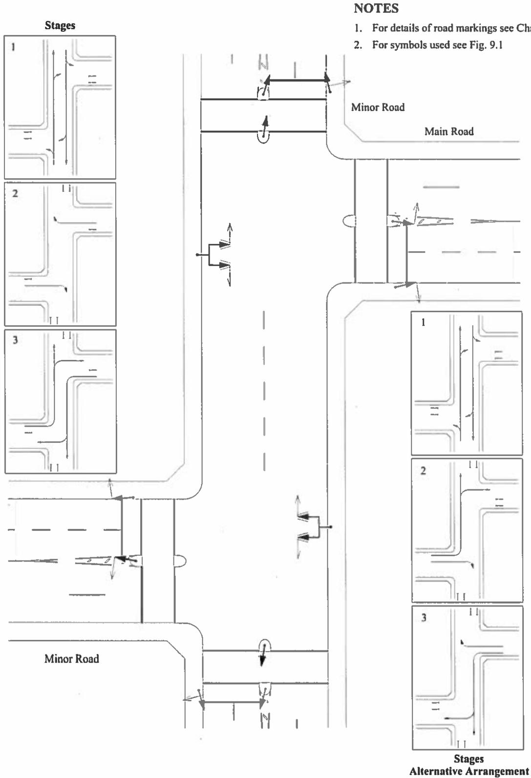
FIG. 9.7 Signal Layout at Left / Right Stagger
