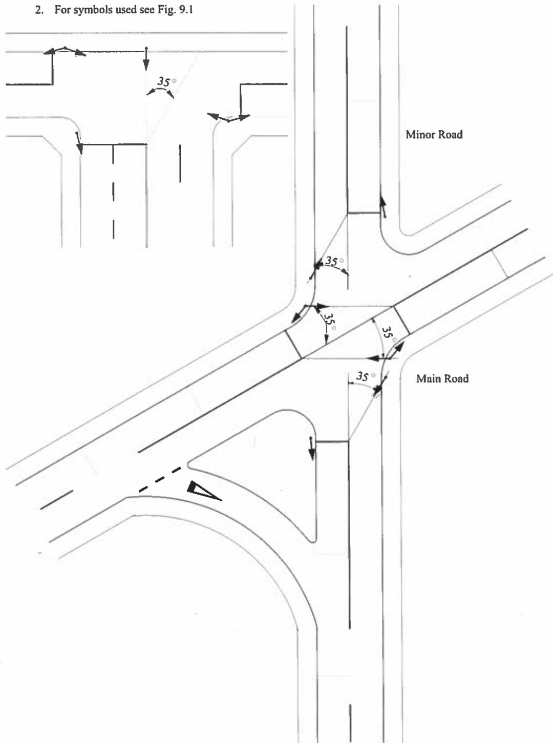
FIG. 9.11 Signals Layout Showing Positioning of Secondary Signals
