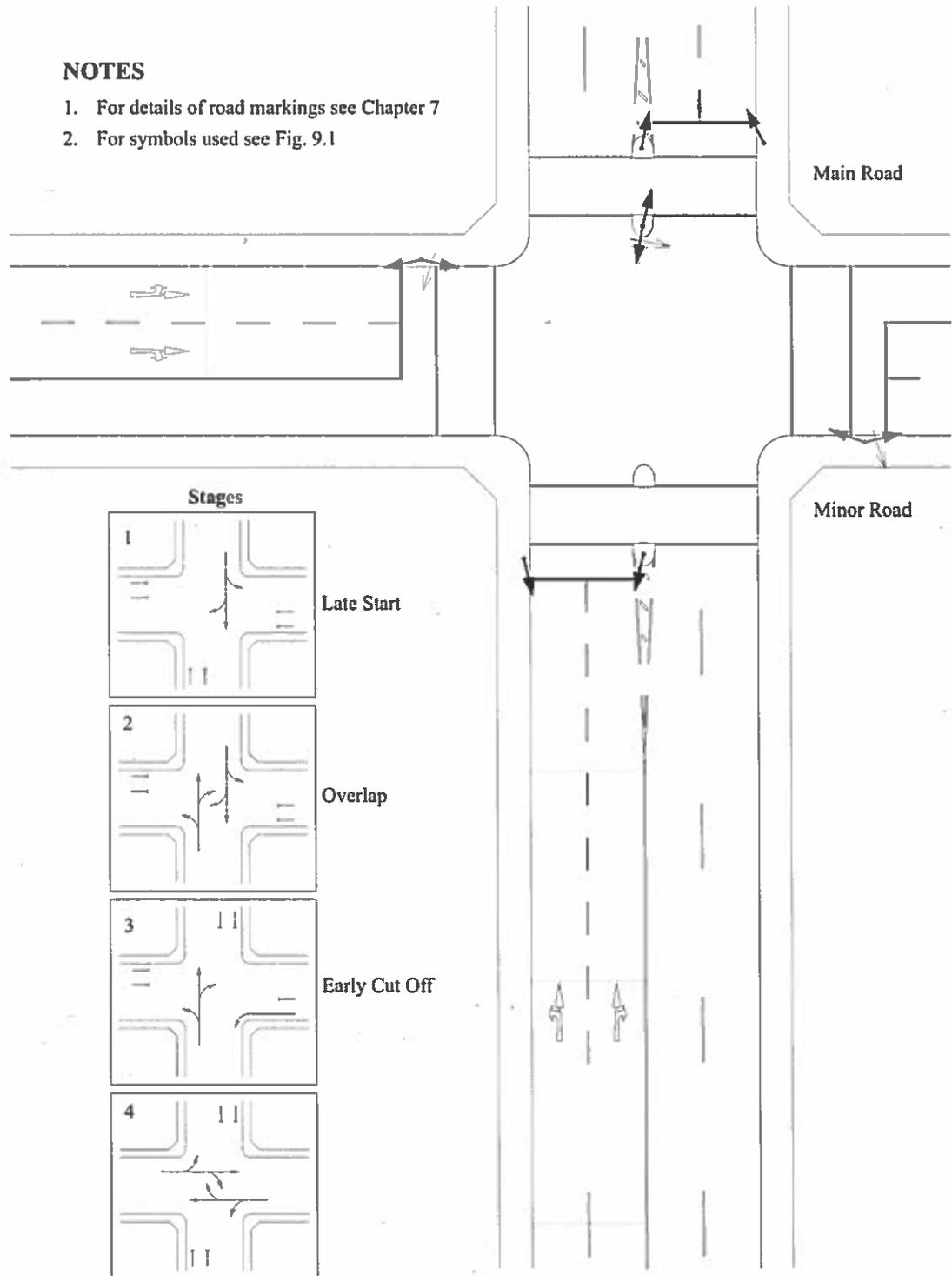
FIG. 9.9 Staging Arrangement for Late Release, Early Cut-off and Filter
