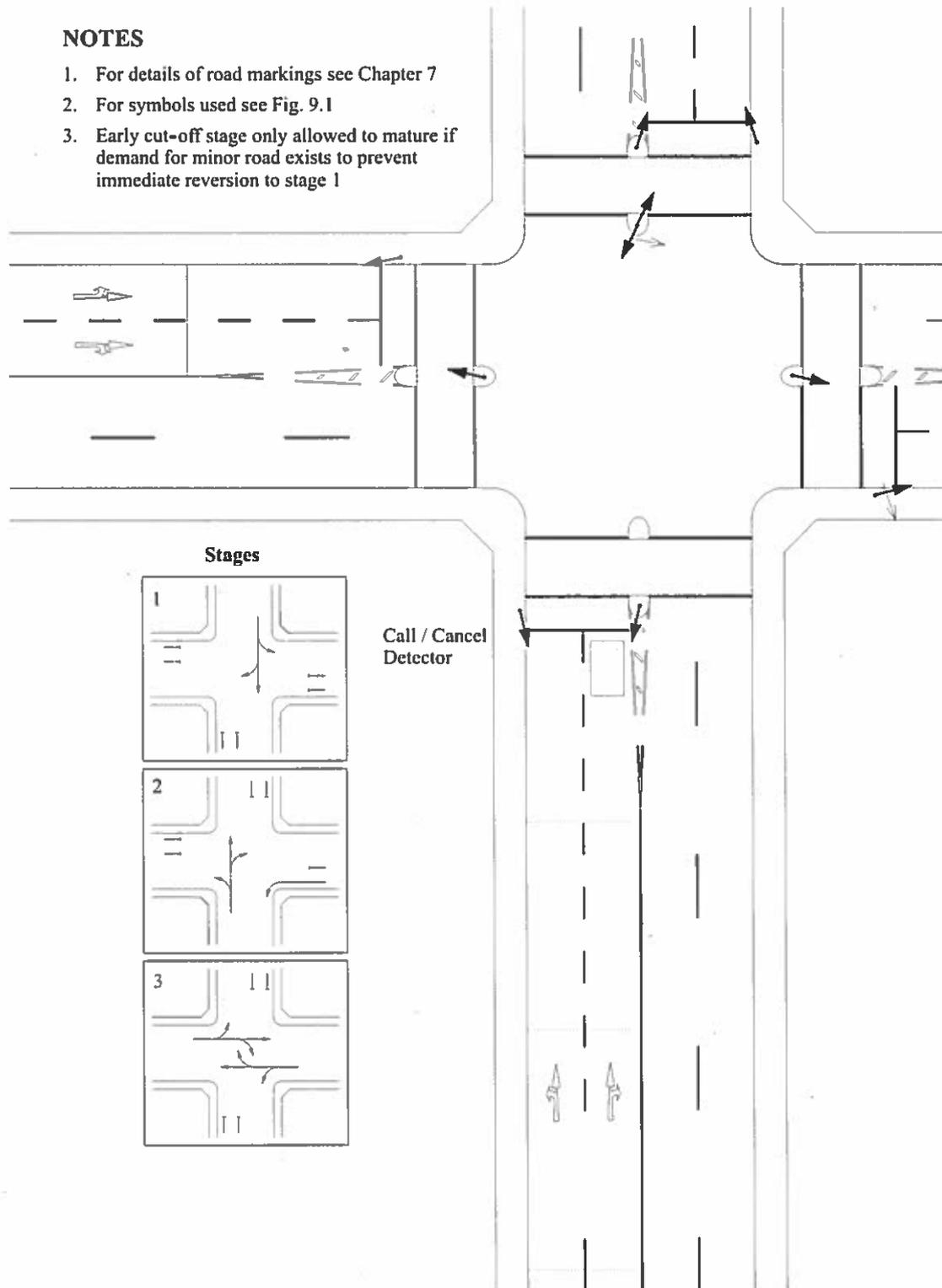
FIG. 9.10 Signal Layout with Early Cut-off Stage
