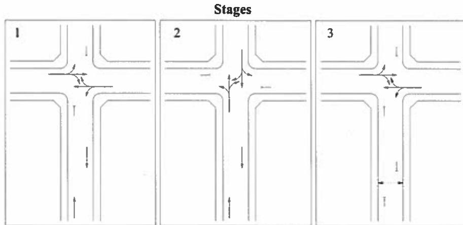
**FIG. 9.14 Displaced Pedestrian Facility**
