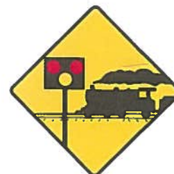
Figure 6.40 Level Crossing Ahead With Lights And Barriers.
