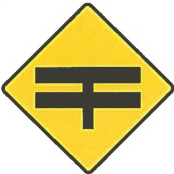
Figure 6.15 T - Junction With Dual Carriageway.
