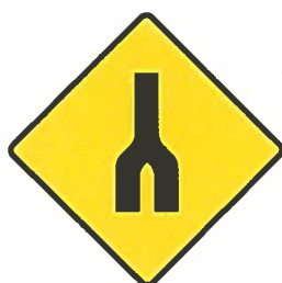
Figure 6.29 Dual Carriageway Ends.
