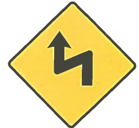
Figure 6.22 Series of Dangerous Corners Ahead.
