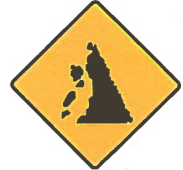
Figure 6.60 Danger of Falling Rocks.
