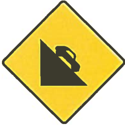
Figure 6.32 Steep Descent Ahead.
