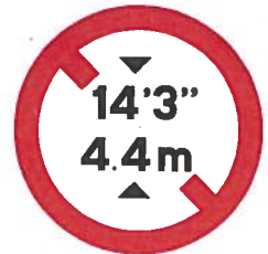
Figure 5.44 Height Restriction Sign
