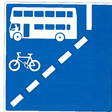
Figure 5.49 Advance Sign For With Flow Bus Lane
