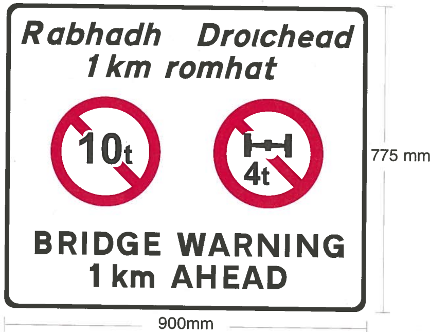
Figure 5.38 Advance Sign Indicating Restriction Ahead
