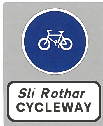
Figure 5.30 Commencement Of Cycleway
