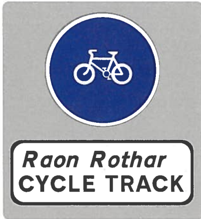
Figure 5.28 Commencement Of Cycle Track
