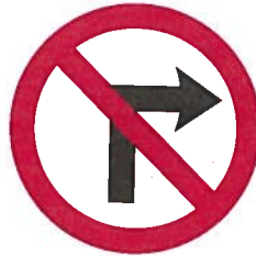
Figure 5.14 NO RIGHT TURN Sign
