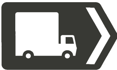
Figure 4.2 Alternative Route For High Vehicles Sign
