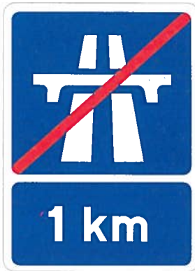
Figure 3.26 End Of Motorway 1km
