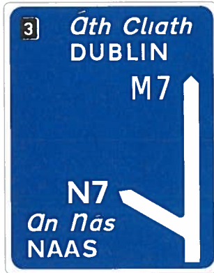
Figure 3.1 Advance Direction Sign
