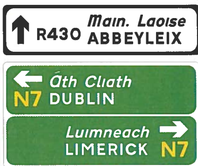
Figure 1.6 Stack Type Advance Direction Sign (Information)
